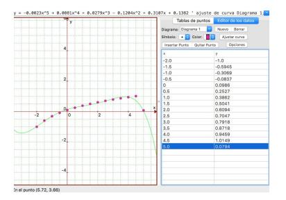
Equation:  $y = -0.0023x^{5} + 0.0081x^{4} + 0.0279x^{3} - 0.1204x^{2} + 0.3107x + 0.1382$ Velocity:  $y = 0.0115x^{4} + 0.0324^{3} + 0.0837x^{2} - 0.2408x + 0.3107$ Acceleration:  $y = 0.046x^{3} + 0.0972x^{2} - 0.2408$
