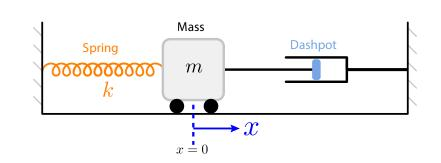
Consider the spring-mass-dashpot system in which m = 1 (kg), and k = 16 (Newton per meter). The position x(t) (meters) of the mass at t (seconds) is governed by the DE
